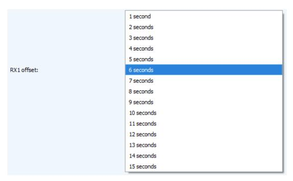
**Join accept delay 1** (not displayed in the "Simple" mode) – sets the time that the device will open the first receiving window to receive confirmation for the join request from the LoRaWAN network. The second window always opens after 1 second after the first.
