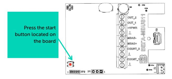
**2. OTAA.** After pressing the start button, the device makes three attempts to connect to the network within the set frequency plan. After the activation in the LoRaWAN network is confirmed, the device sends a signal (LED flashing for 5 seconds) and switches to the "Active" mode. If all attempts fail, the converter will continue to accumulate data and will attempt to connect to the network every 6 hours.
