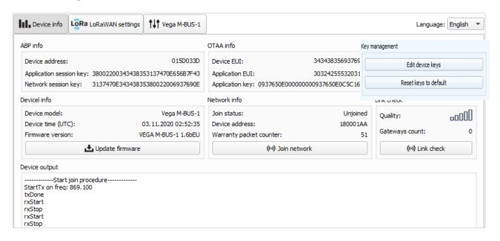
**ABP info** - displays the data necessary to register the device in the LoRaWAN network with ABP method (Activation By Personalization).
