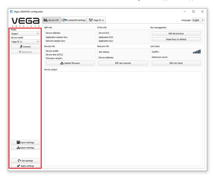
The left side menu allows you to switch between the "Simple" and "Expert" operating modes, select a device model, connect to, or disconnect from a device.
