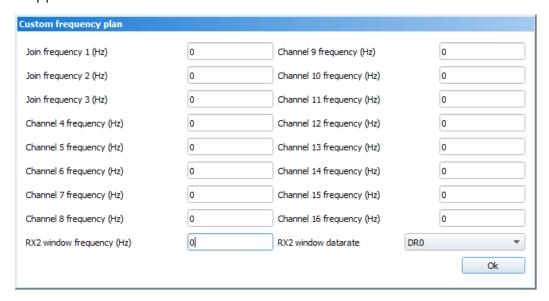
This frequency plan allows you to set up to 16 channels, as well as the frequency and speed of the second receiving window.
