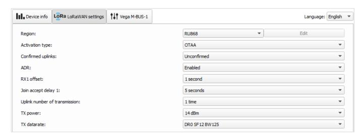
Region - allows you to select one of installed frequency plans or specify a custom frequency plan. Custom frequency plan is EU-868 based.
