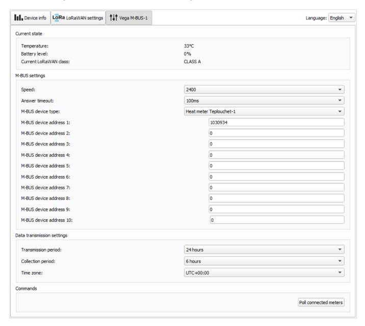
**Current state** – displays the current parameters of the device - the internal temperature of the device, the battery level and the current LoRaWAN class.
